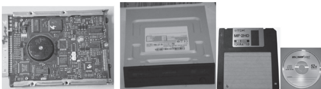
Figure 1.34 | Storage devices (i) Hard disk drive, (ii) DVD drive, (iii) Floppy disk, (iv) CD
